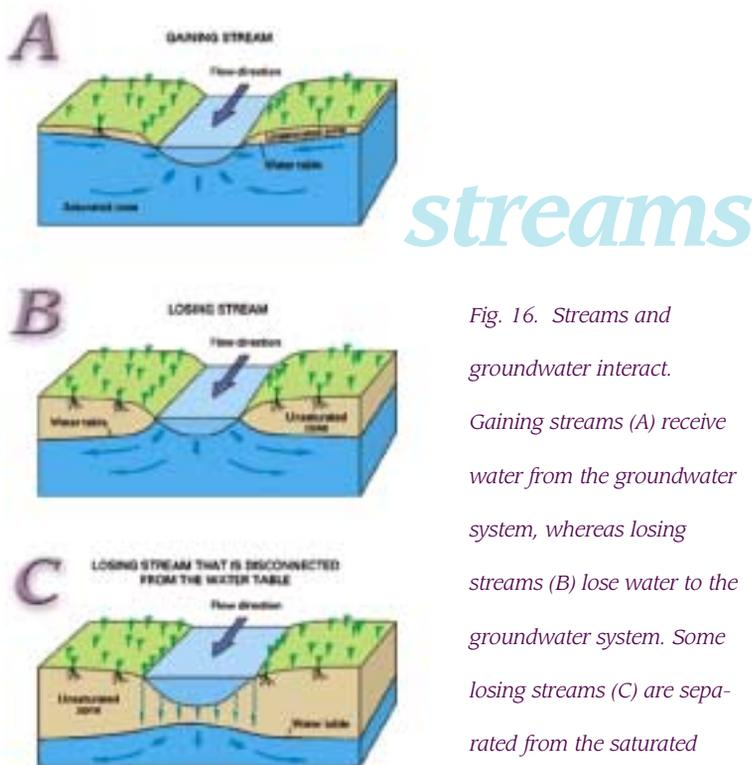
Fig. 16. Streams and groundwater interact. Gaining streams (A) receive water from the groundwater system, whereas losing streams (B) lose water to the groundwater system. Some losing streams (C) are separated from the saturated groundwater system by an unsaturated zone.
