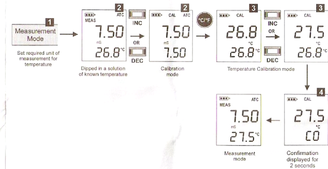
Figure 10: Temperature calibration sequence
