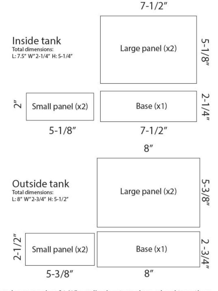
Panels are made of 1/8" acrylic sheets and are glued together using acrylic glue of strength 4.
